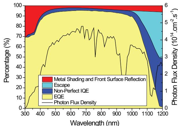
**Figure 4.** Optical loss analysis of the best cell shown in **Figure 3**. The dark blue region indicates recombination and parasitic absorption losses, and the red region indicates the optical loss due to front-surface reflection and metal shading. The loss analysis assumes an AM1.5G illumination spectrum, the photon flux of which is shown superimposed on the EQE data.
