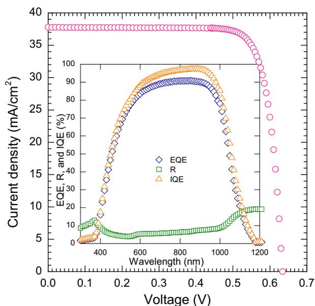
**Figure 3.** Measured light  $J$ - $V$  behavior of the best cell measured under standard one sun conditions. The inset shows the external and internal quantum efficiencies accompanied by the measured reflectance for the cell.
