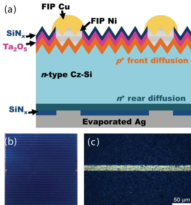
**Figure 1.** a) Schematic representation of front-junction  $p^+nn^+$  silicon solar cell with front ALD  $Ta_2O_5$ /PECVD  $SiN_x$  ARC and rear PECVD  $SiN_x$  surface passivation; Optical microscope images of (b) a completed solar cell, and (c) a laser-ablated front finger opening.
