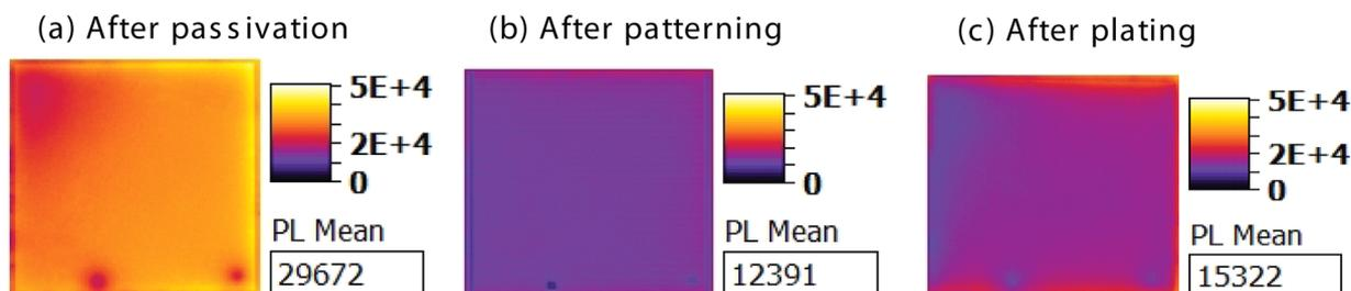
**Figure 2.** Open circuit PL images of the solar cells processed after (a) surface passivation, (b) laser patterning, and (c) field-induced plating.
