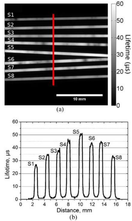
Fig. 3. (a) PL calibrated lifetime image of silicon strips after being detached from the wafer frame and flipped by  $90^\circ$ . The images were taken with incident photon flux of  $2.7 \times 10^{18} \text{ cm}^{-2} \cdot \text{s}^{-1}$ . (b) Line scan of the lifetimes across various silicon strips.
