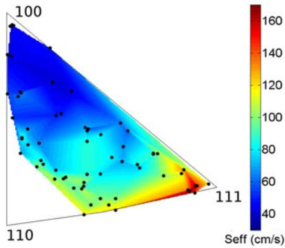
Fig. 7. Interpolated result of the surface recombination velocity of each orientation plotted in an IPF based on measured grains, represented by dark dots.
