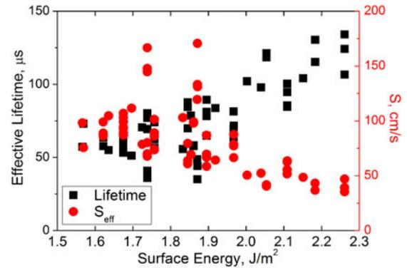
Fig. 6. Effective lifetimes and surface recombination velocities of individual grains in the studied mc-Si wafers classified according to their corresponding surface energies.
