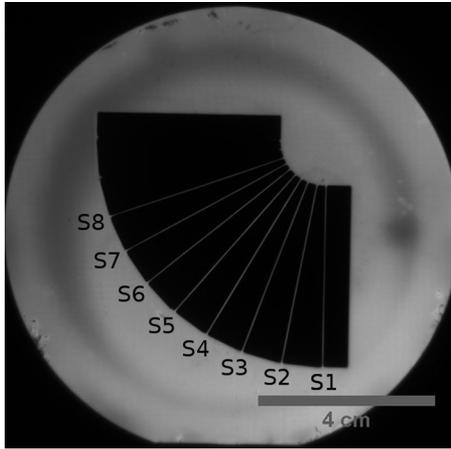
Fig. 2. PL image of silicon strips before being detached from the monocrystalline silicon wafer frame.
