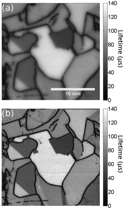
Fig. 5. PL calibrated lifetime images (a) before and (b) after applying the carrier desmearing technique. The images were taken with an incident photon flux of  $2.7 \times 10^{18} \text{ cm}^{-2}\cdot\text{s}^{-1}$ .
