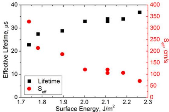
Fig. 4. Effective lifetime and surface recombination velocity of each studied silicon strip classified according to its corresponding surface energy.
