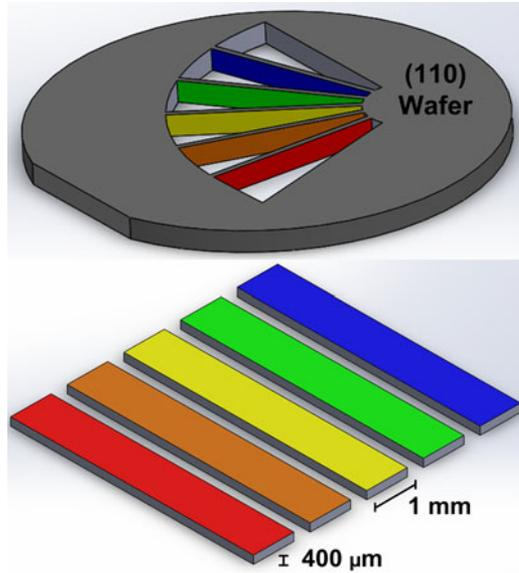
Fig. 1. Silicon strips created from a (1 1 0)-oriented monocrystalline silicon wafer through laser cutting. Note that the diagram is not to scale for visual illustration purposes.
