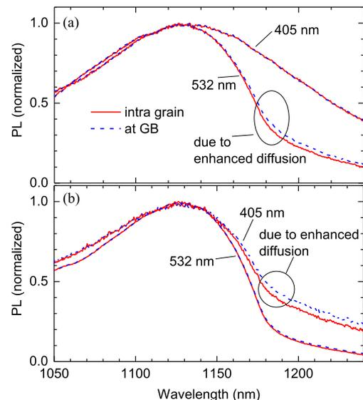
Fig. 5. Comparison of normalized PL spectra between 532- and 405-nm excitation lights at a GB and in the intragrain region, measured at room temperature. (a) Sample 2, heavy phosphorus diffusion with a sheet resistance of  $10 \Omega/\square$ . (b) Sample 4, light phosphorus diffusion with a sheet resistance of  $120 \Omega/\square$ .
