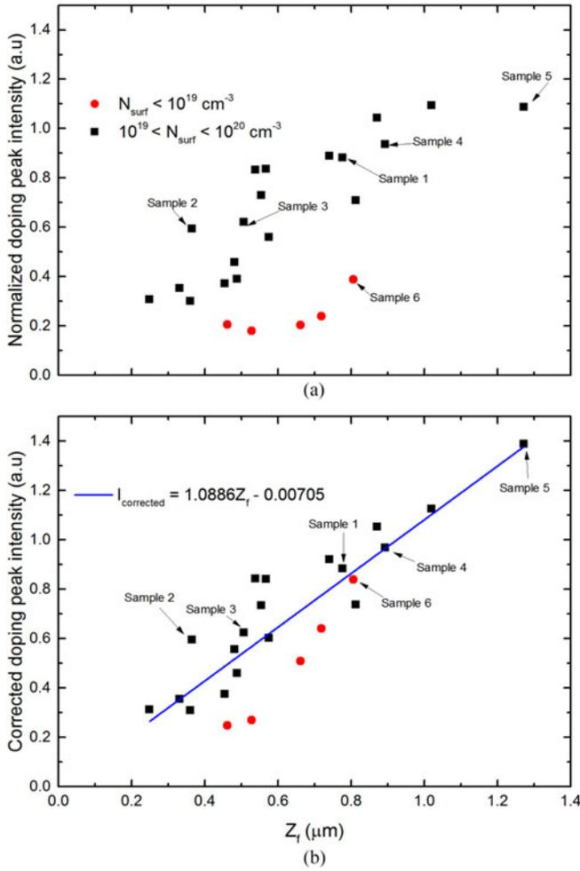
Fig. 3. Normalized doping peak intensity as a function of depth factor, (a) without any correction, and (b) including a correction for the effect of incomplete ionization on PL intensity. Representative samples shown in Fig. 2 are also labeled accordingly.
