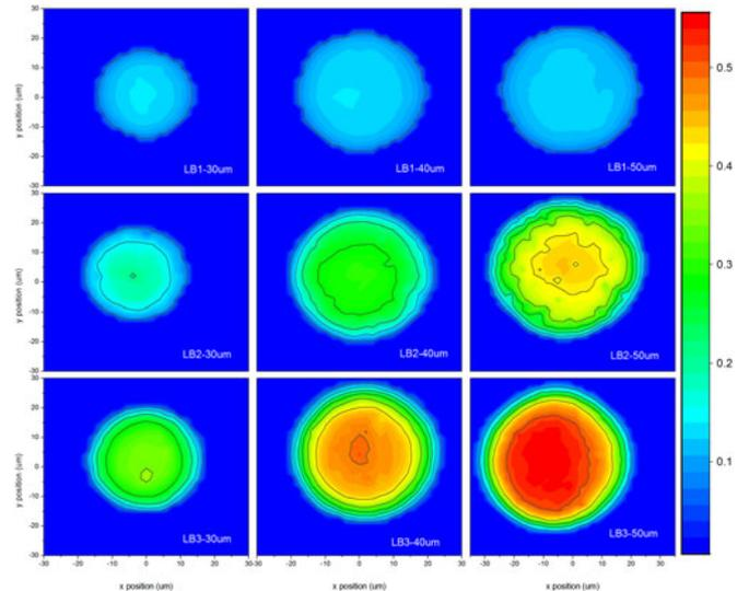
Fig. 7. 2-D scanned maps of  $z_f$ , for locally diffused samples through 30, 40, and 50  $\mu\text{m}$  dielectric mask openings.
