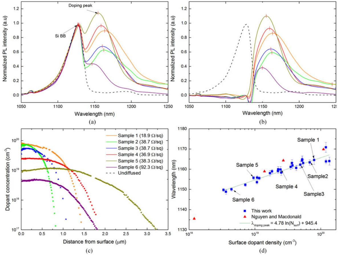
Fig. 2. (a) Normalized PL spectra of a selection of boron-diffused samples with different doping profiles, measured with a 532 nm laser at 79 K. (b) Modified PL spectra by subtracting PL spectra of undiffused Si. (c) The corresponding doping profiles with sheet resistances. (d) Measured wavelengths of the doping peaks as a function of  $N_{\text{surf}}$  for all samples, along with Nguyen and Macdonald's results [9] measured from homogeneously heavily boron-doped silicon.
