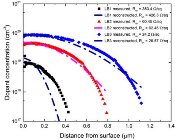
Fig. 5. Measured and reconstructed doping profiles, used for localized diffusions, with corresponding sheet resistances.
