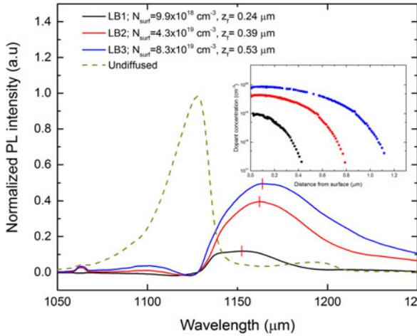
Fig. 4. Normalized and subtracted PL spectra of locally diffused samples, labeled as LB1–3 with  $N_{\text{surf}}$  and  $z_f$ , measured at the center region of diffused  $1 \text{ cm} \times 1 \text{ cm}$  with a 532 nm laser at 79 K. The corresponding profiles are shown in the inset.
