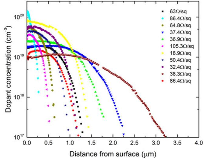
Fig. 1. Doping profiles measured by ECV for a selection of thermally boron-diffused samples used for  $\mu$ -PLS analysis, with corresponding measured sheet resistances.
