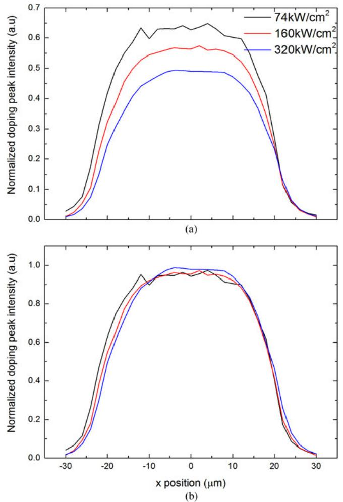
Fig. 8. (a) Horizontal section of 2-D map of LB3- $40\ \mu\text{m}$  sample's doping peak intensity, measured with different excitation intensity ( $74$ ,  $160$ ,  $320\ \text{kW}/\text{cm}^2$ ), and (b) normalized to 1 for the comparison.
