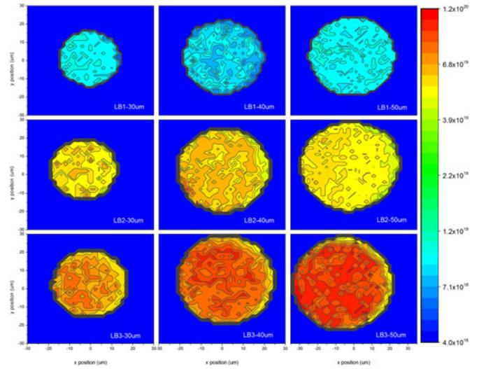
Fig. 6. 2-D scanned maps of  $N_{\text{surf}}$ , for locally diffused samples through 30, 40, and 50  $\mu\text{m}$  dielectric mask openings.
