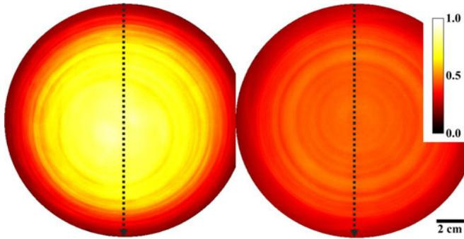
Fig. 6. Relative doping images calculated from bulk lifetime and PL counts for samples N80 (left) and N674 (right), both plotted on the same relative color scale. The dotted lines denote the positions of cross-section shown in Fig. 7.
