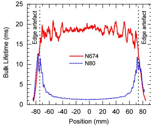
Fig. 4. Cross-sectional bulk lifetime profiles for samples N80 and N674. Vertical lines positioned toward the left and right edge of the cross-section indicate the measurement artefact caused by the surfaces toward the periphery of the discs.
