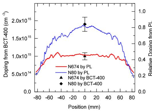
Fig. 7. Cross-sectional doping profiles for samples N80 and N674. The relative doping from PL is calibrated using the average of resistivity measurements from a Sinton Instruments BCT-400 in a central location on N80. Error bars for the BCT-400 measurements are based on repeated measurements.
