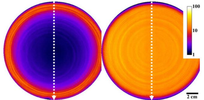
Fig. 3. Bulk lifetime images of sample N80 (left) and N674 (right). The color scale represents bulk lifetime in milliseconds and is mapped to lifetime logarithmically. Dotted lines represent the position of the cross-sections. Note that the samples are slightly larger than the field of view of the PL system.
