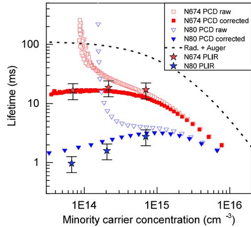
Fig. 5. Injection-dependent lifetime for samples N674 and N80 from transient photoconductance decay (PCD) measurements. Both raw data (open symbols) and trapping corrected data (solid symbols) are presented. Bulk lifetimes from PLIR are shown at three injection levels with errors bars based on an estimated uncertainty of the technique. The Auger and radiatively limited lifetime is also shown.
